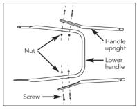
Proceed to inserting the two handle uprights into the upper handle.
