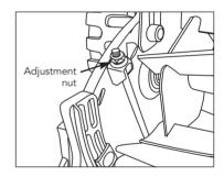
To tighten the blades, or move them closer against the cutting bar, tighten both cutting bar adjustment nuts equally turning them clockwise. If the mower is only cutting on one side, the cutting bar may be out of alignment with the blade reel. Therefore, tighten the side of the mower that is not cutting to bring it back into alignment.
